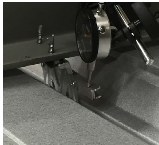
Figure 15: Rotational-Lateral Stiffness Test Configuration
