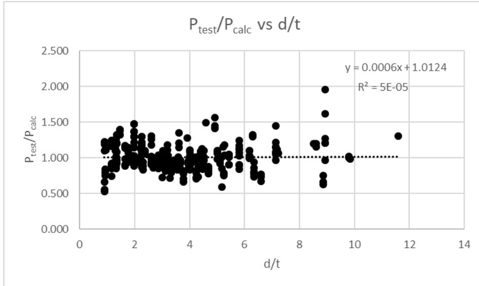
Figure 4.5 P<sub>test</sub>/P<sub>calc</sub> (with adjustment factor) versus d/t
