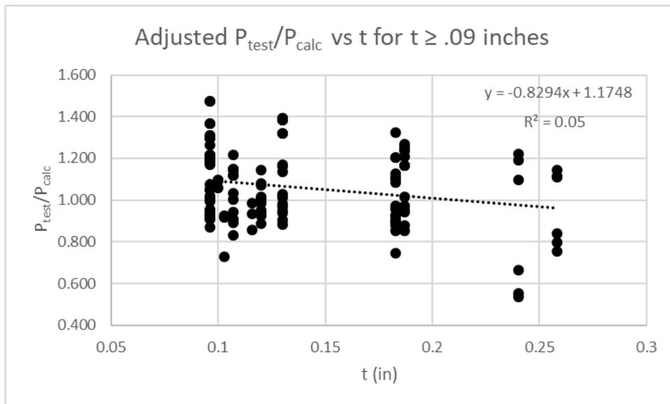
Figure 4.11 Adjusted P<sub>test</sub>/P<sub>calc</sub> versus t for t ≥ 0.09 inches
