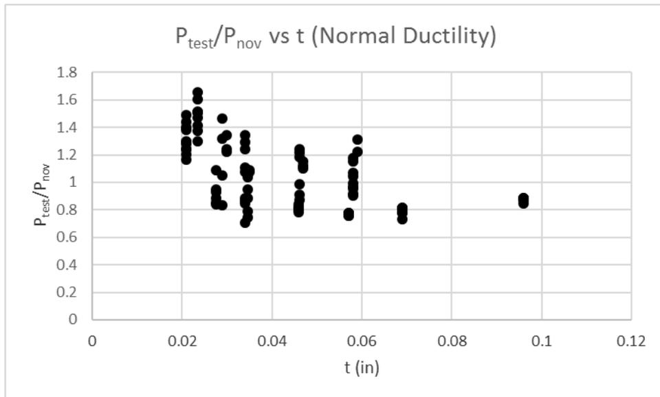
Figure 3.2 – Tested strength to nominal strength ratio versus thickness for ductile
