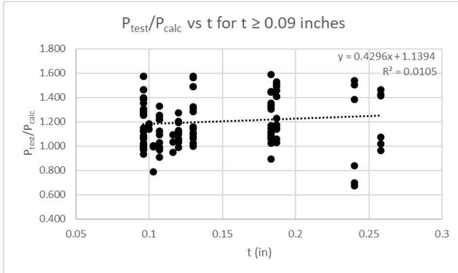
Figure 4.10 Original P<sub>test</sub>/P<sub>calc</sub> versus t for t ≥ 0.09 inches
