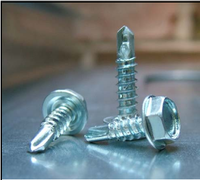
Zinc plated hex washer head (HWH) self-drilling screws (SDS) are the most common type used for steel-to-steel connections when sheathing will not be applied over the fastener head. When sheathing will be applied, a low-profile head (such as pan-head or modified truss head) is more commonly used.
