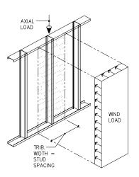
The basis for consideration of these three conditions stems from the language contained in Section 1609.6.2.3 of the 2000 International Building Code: "Members that act as both part of the main force resisting system and as components and cladding shall be designed for separate load cases."
