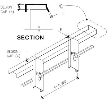
$\begin{array}{l} b_{eff} = 0.11 \; x \; (\; e^{0.5} / \; t^{1.5} \; ) + \; 5.5 \; < \; or = S \\ P_n = b_{eff} \; x \; t^2 \; x \; F_y \; / \; 4 \; x \; e \end{array}$
