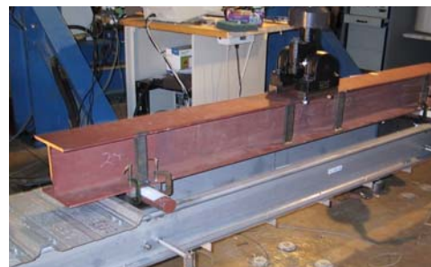
Fig. 1 Four point bending test setup
