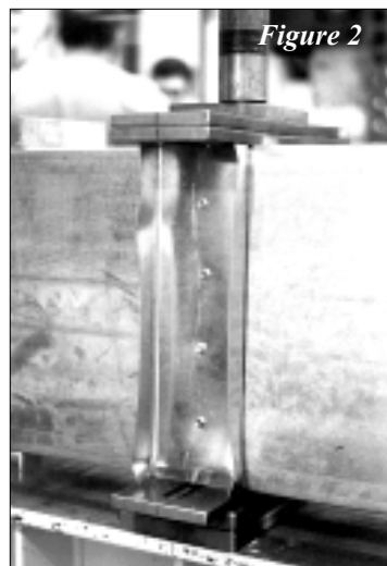
Failure of End-Outside Stud Stiffener
