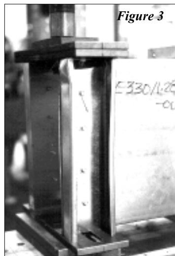
Failure of Interior-Outside Track Stiffener
